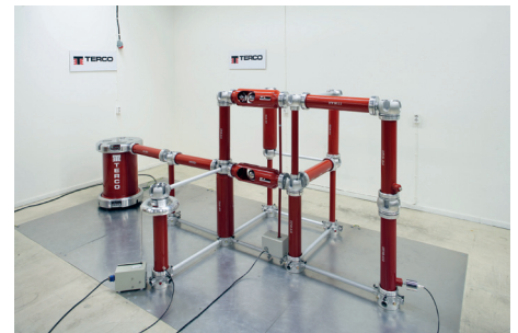
2-stage Impulse Voltage Test Set-up
