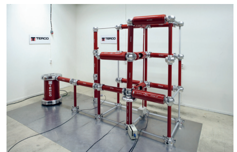
3-stage DC Voltage Test Set-up
