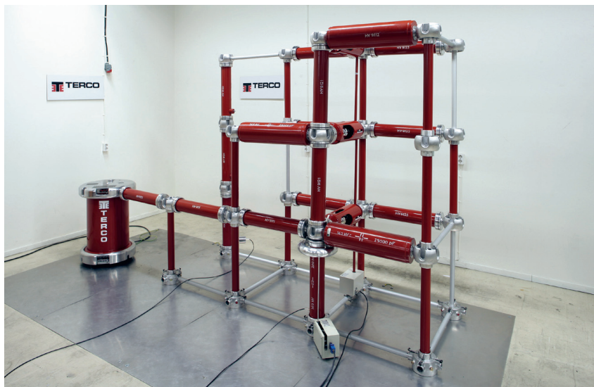
3-stage Impulse Voltage Test Set-up
