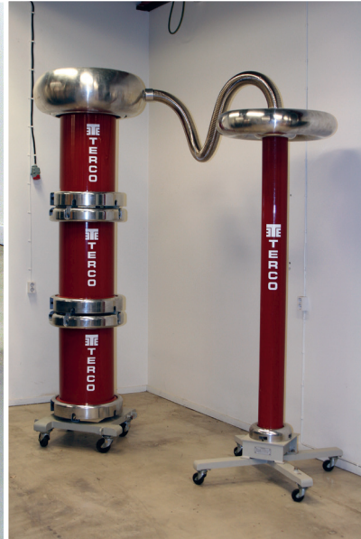
3-stage AC Voltage Test Set-up
