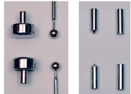
Flat and 20 mm Sphere Electrodes
